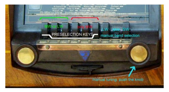
NOTE 1: for manual tuning, push one of the last three keys (first: LW; second: MW; third: SW), then push the tuning knob until it locks; finally, to change stations, turn the tuning knob. The subsequent activation of one of the first six preselection keys causes the release of the manual tuning knob.
